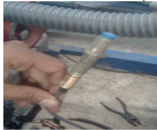
Figure 3. The proximity sensor that is used in the 4 stroke single cylinder petrol engine
