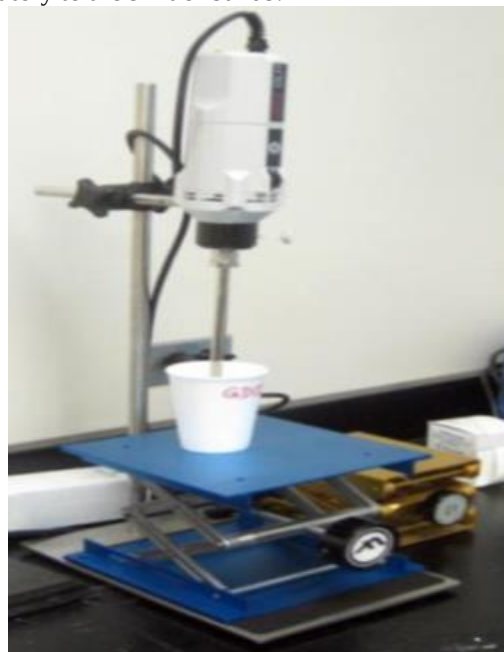
Figure 3. Probe type ultra sonicator was used for homogeneous mixing of nanoclay with the modified polymer.
