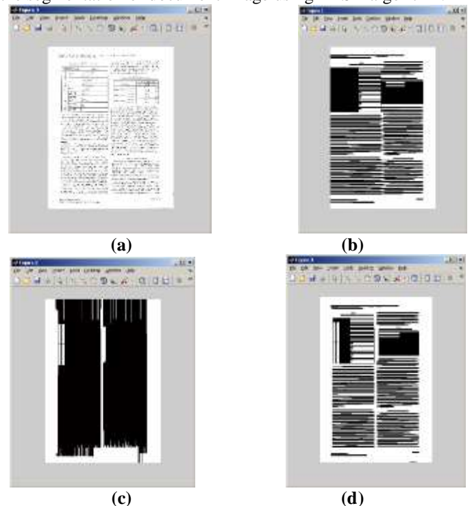
Fig 2. (a) Original document image. (b) Result of horizontal smearing. (c) Result of vertical smearing. (d) Final result of segmentation
