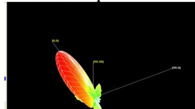
Fig .4.3 Radiation Pattern for 4x1 Patch Array
