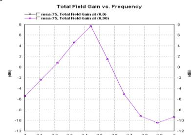
**Fig. 4.2 Gain vs Freq for 4x1 Patch Array**
