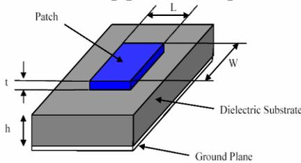
Fig. 1.2 : Microstrip patch Antenna
