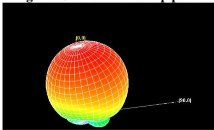
**Fig 2.5 Radiation pattern of single patch antenna**
