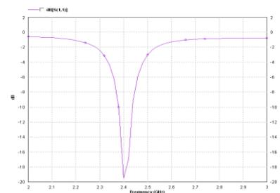
Fig.2.2 Return loss curve for Microstrip Patch
