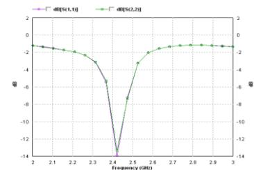
**Fig. 4.1 Return loss for 4x1 Patch Array**
