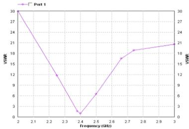
**Fig 2.3 VSWR vs Freq curve for Microstrip Patch**
