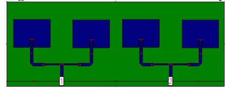
**Fig. 3.2 Geometry of 4x1 antenna array**
