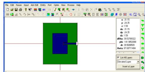
Fig.2.1 Geometry of Microstrip Patch
