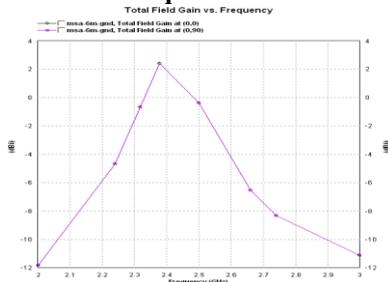
**Fig. 2.4 Gain of Microstrip patch**
