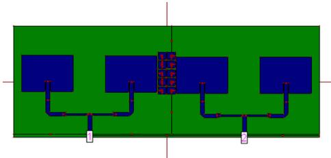
Fig 6.1 4X1 Microstrip Antenna Array with EBG
