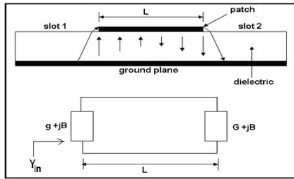
Fig. 1.1 : Microstrip patch and equivalent circuit
