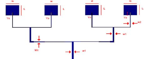
**Fig.3.1 Feed network for antenna array**
