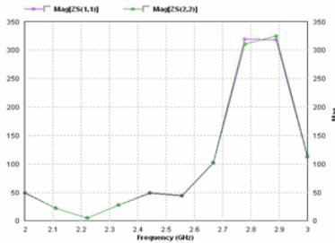
Fig .4.4 Magnitude of Impedance for 4x1 Patch Array Surface Wave Propagation and Mutual Coupling
