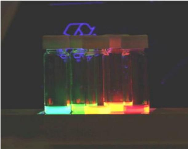
a) Electron micrograph of (anatase) titanium dioxide ( $\text{TiO}_2$ ) nanoparticles; b) Colloidal quantum dots irradiated with a UV light. Different sized quantum dots emit different color light due to quantum confinement
