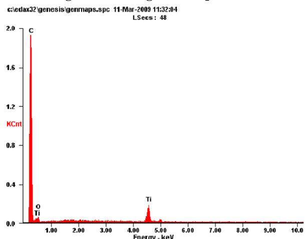
Fig 3. EDX image of  $\text{TiO}_2$ -MWNTs
