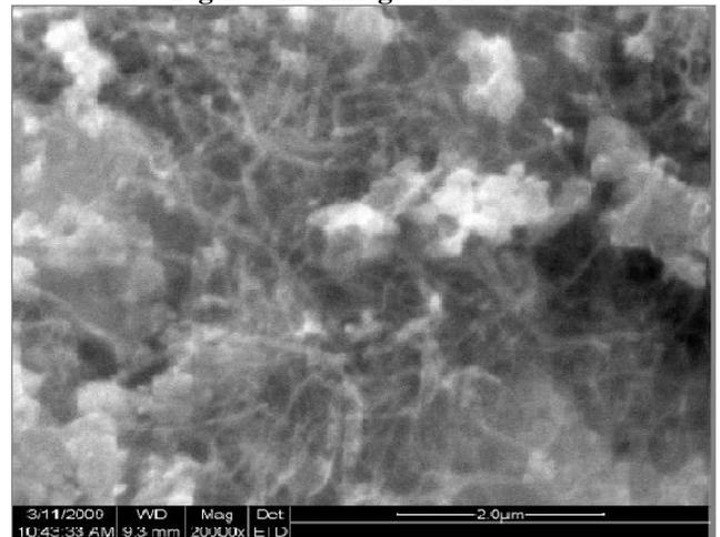
Fig 2. SEM images of  $\text{TiO}_2$ -MWNTs
