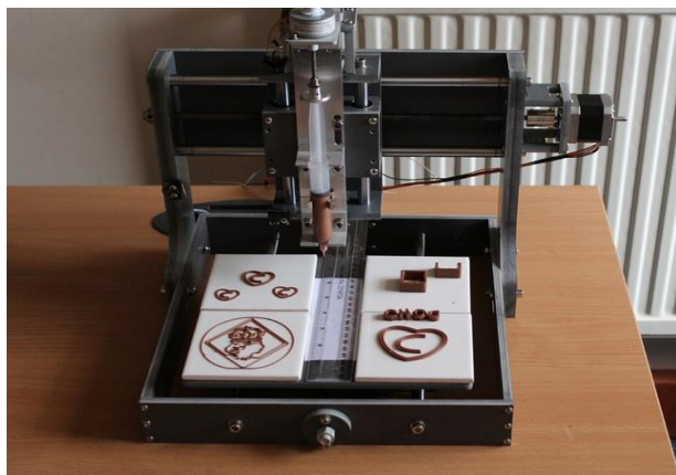
Figure 7. 3d printer using chocolate pastes as a material for printing
