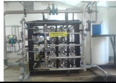
Figure 5 Reverse Osmosis Plant Stage I and II
