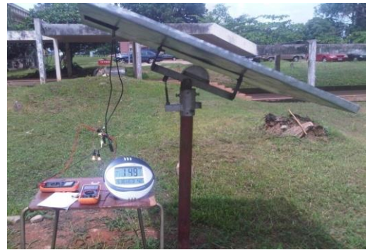
Figure 1. Optimal tilt angle measurement for solar panel Results and Discussion
