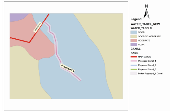
Fig 16. GWP ZONE MAP (Buffer Analysis of Proposed-I Canal) OF SOMNALA MINOR IRRIGATION SCHEME
