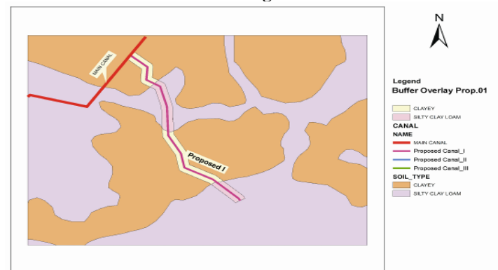
Fig 12. SOIL MAP (Buffer Overlay Intersect Analysis of Proposed-I Canal) Somnala Minor Irrigation Scheme
