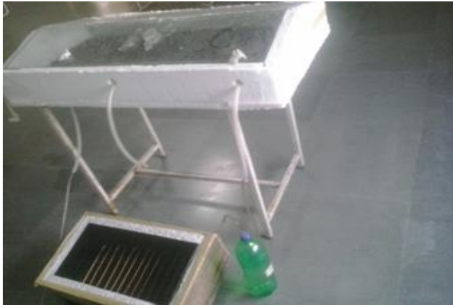
Fig 1. Experiment Setup of double slope glass active solar still
