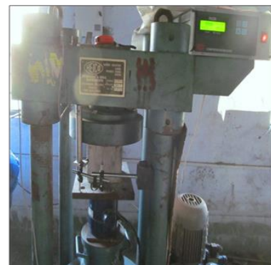
Fig 2. Testing set-up, Cube Specimen for Compressive Strength
