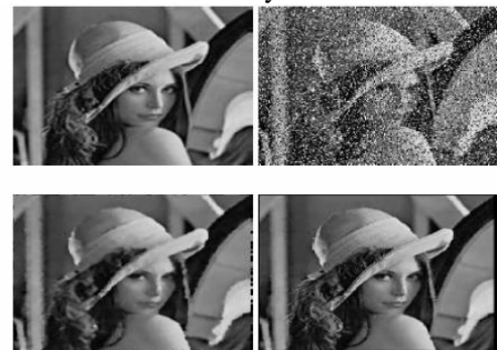
Fig.7 Results of filtering with adaptive median filter and adaptive rank order filter. First row : Original image, noisy image; Second row : Adaptive median filter, Adaptive Rank Order filter
