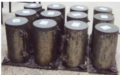
a) 18 casted test cylinders before curing
