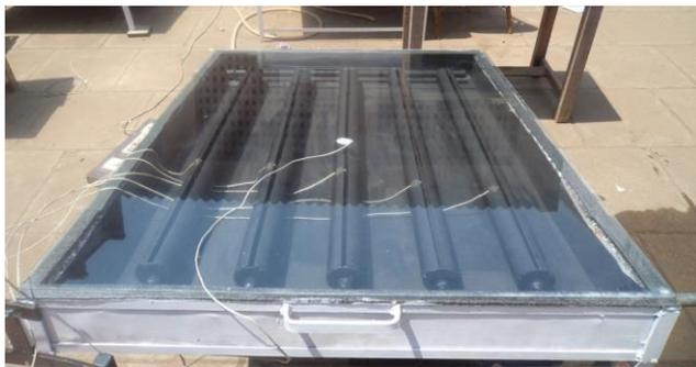
**Figure 4. Experimental setup of a solar circular cavity receiver**
