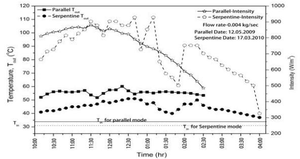
Figure 11. Comparison between parallel and serpentine mode of flow
