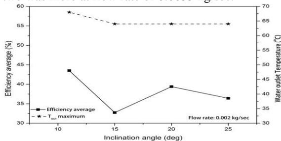
Figure 10. Efficiency and  $T_{out}$  comparison for different inclination angles
