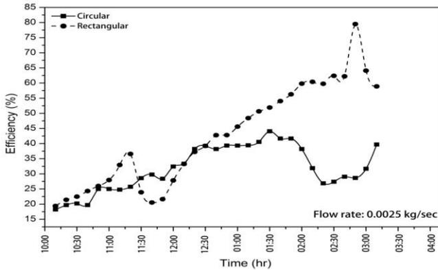
Figure 8. Variation in efficiency with respect to circular and rectangular cavities
