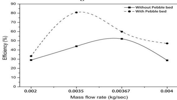
Figure 9. Effect of pebble bed on the performance of cavity collector
