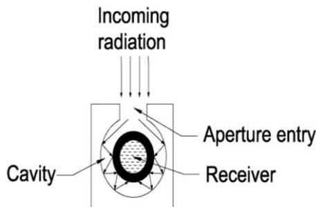
Figure 2. Multi reflection process of a solar cavity collector
