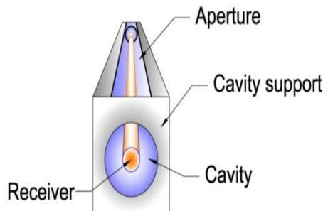
Figure1. Detailed view of a single cavity tube
