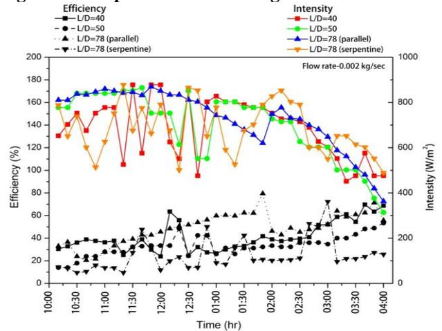
**Figure 7. Effect of L/D ratio on the performances of solar cavity collector**
