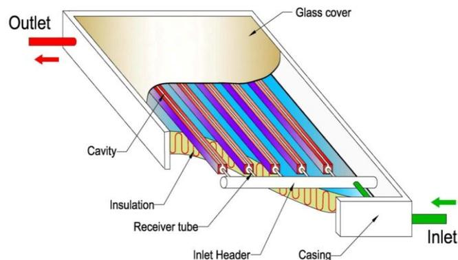
**Figure 5. Schematic diagram of a flat plate cavity collector**
