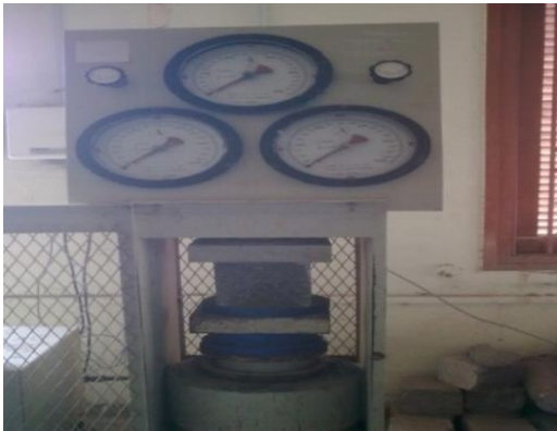
Fig 4. Specimen in compressive testing
