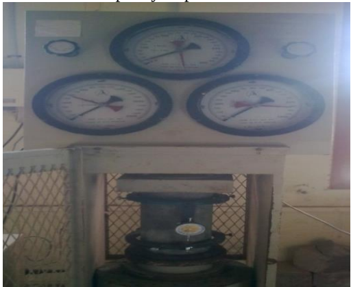
Fig 6. Specimen in compressive testing
