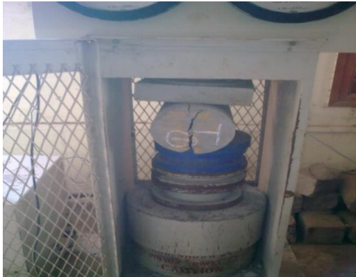
Fig 10 . Specimen in compressive testing
