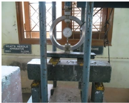
Fig 12. Specimen in flexural testing
