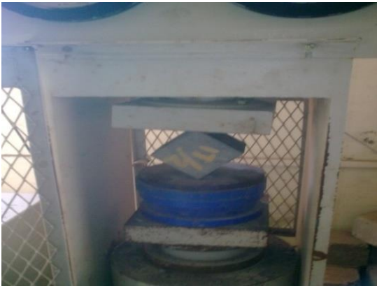
Fig 8. Specimen in compressive testing
