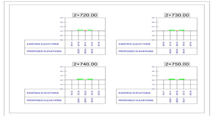
Fig 6. Cross-sections of the Proposal I Canal Alignment at the interval of 10m.
