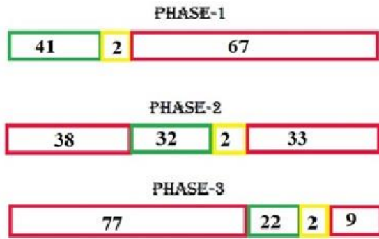
FIG 7.7. Signal Phase Diagram for Evening Session
