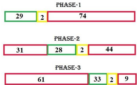
Fig 7.5. Signal Phase Diagram for Afternoon Session. 7.4 Calculation of Cycle length for Evening Session
