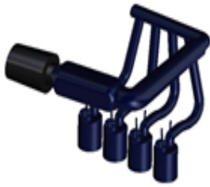
Fig 3. Solid model of modified air intake system rectangular cross section.
