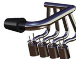
Fig 2. Solid model of modified air intake system circular cross section.
