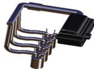
Fig 1. Solid Model of existing air intake system
