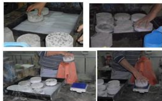
Figure 18. Sorptivity test method.
