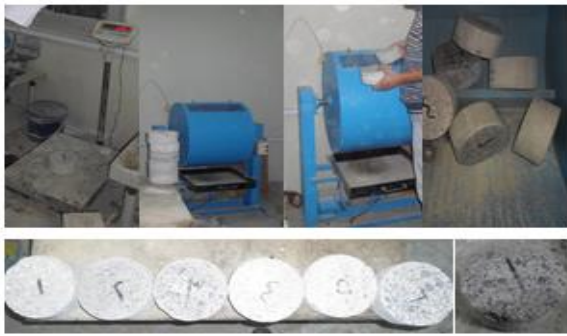
Figure 14. Los Angeles (LA) abrasion machine called Cantabro Test method.
