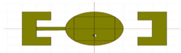
Fig 5. Design of Circular patch antenna with c-shaped slots and switches were connected as ON and OFF condition
