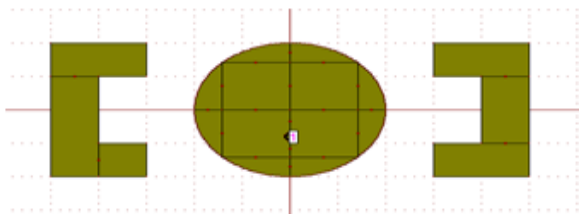
Fig 2. Design of Circular patch antenna with c-shaped slots and two switches are in OFF condition
