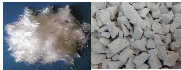
Figure 1. (a)Shown the polypropylene fibers (b) shown the Waste Crushed Thermostone Coarse Aggregate .
