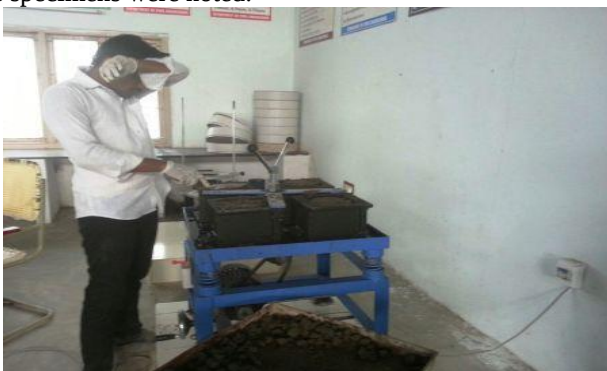
Figure 3. Casting of cubes
