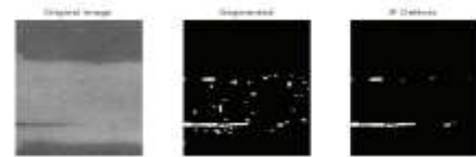
Figure 6. Sample image of incomplete fusion (IF).
