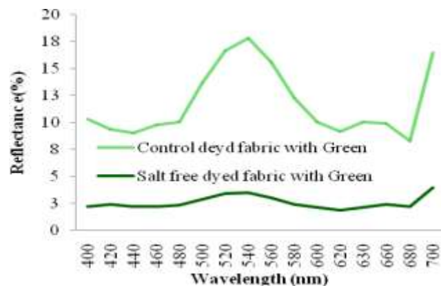
Figure 1. Reflectance curve for control and modified cotton garments dyed without salt.
