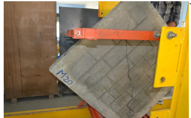
Figure 8. Propagation of crack in the specimen.
