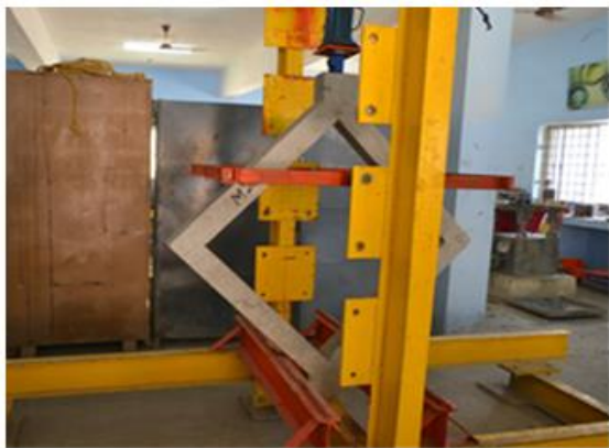
Figure 6. Test setup of specimen in loading frame.
