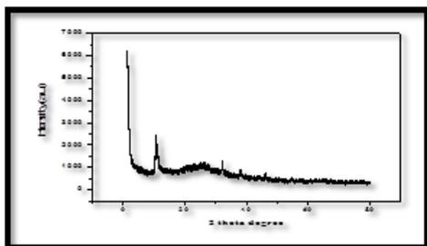
Fig 4. XRD patterns of bio functionalized AgNPs.
