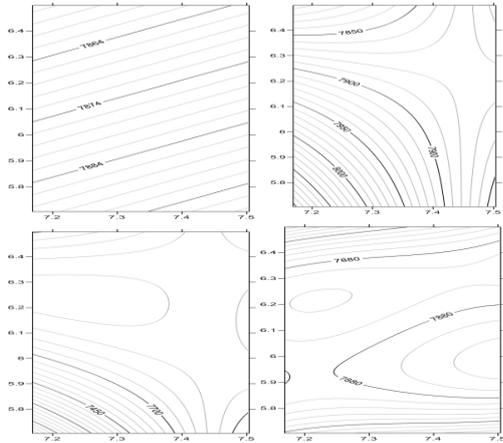
**Fig 4. First to fourth degree (polynomial) surfaces of the Regional fields of the Aeromagnetic data.**
