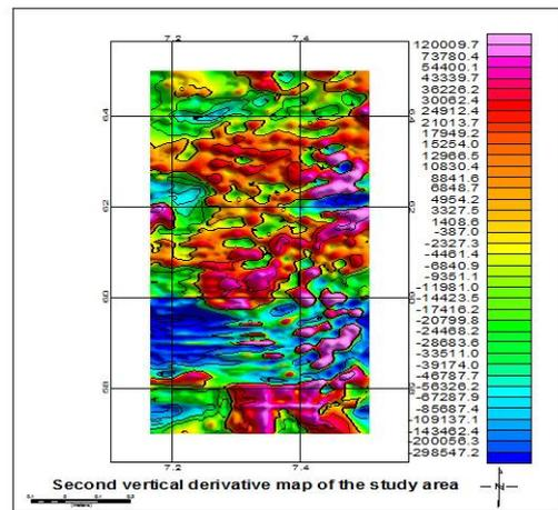
**Fig 7. Second Vertical Derivative of Zero Contour Map of the Study area.**
