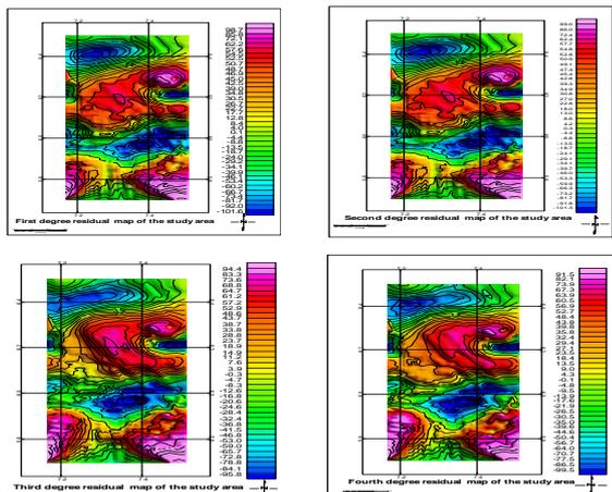
**5. First to fourth degree residual surfaces of the Residual fields of the Aeromagnetic data.**
