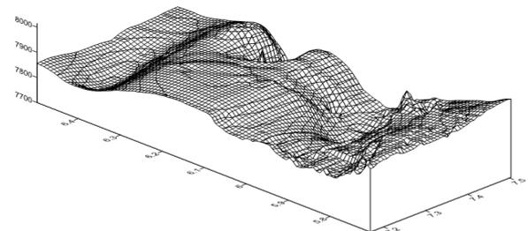
Figure 3. Total field of the aeromagnetic data presented as 3-D map showing the basement topography.
