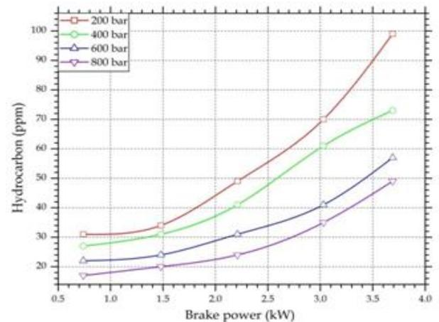
**Fig. 6 Comparison of Hydrocarbon for different fuel injection pressures**
