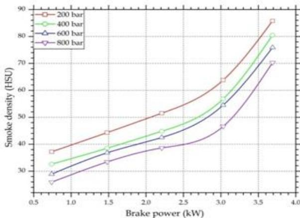
**Fig 4. Comparison of Smoke density for different fuel injection pressures**
