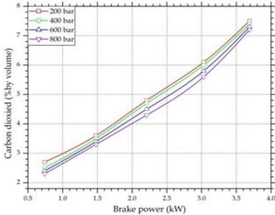
Fig 8. Comparison of Carbon dioxide for different fuel injection pressures
