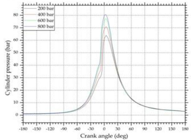
Fig 10. Variation of Cylinder Pressure for different fuel injection pressures
