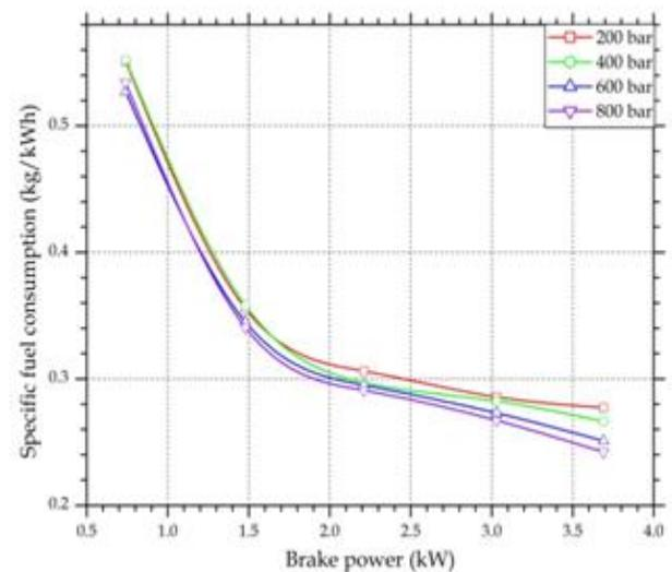
**Fig 2. Variation of SFC for different fuel injection pressures**
