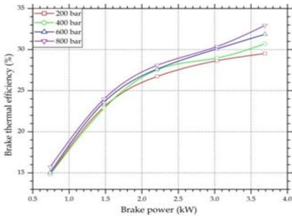
**Fig 3. Variation of Brake thermal efficiency for different fuel injection pressures**
