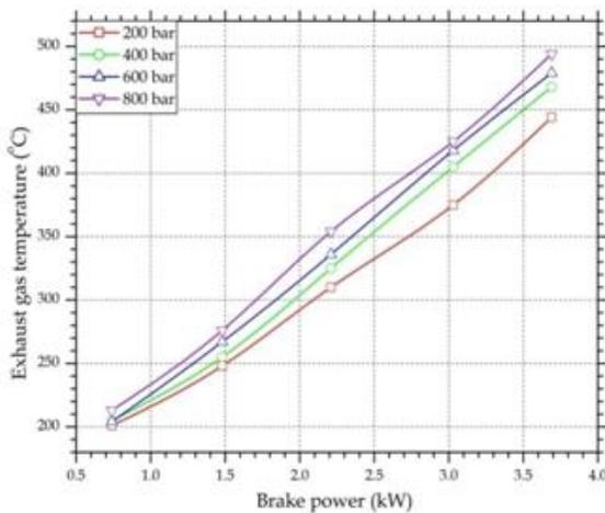
Fig 9. Variation of Exhaust gas temperature for different fuel injection pressures
