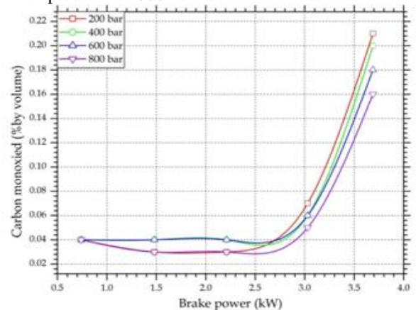
**Fig 7. Comparison of Carbon monoxide for different fuel injection pressures**
