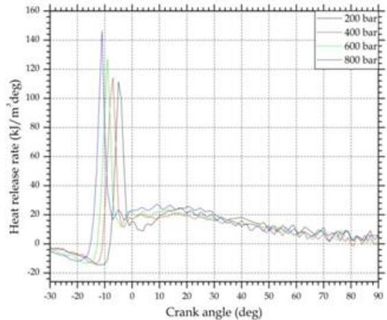
Fig 11. Variation of Heat release rate for different fuel injection pressures
