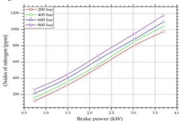
**Fig 5. Comparison of Oxides of nitrogen for different fuel injection pressures**
