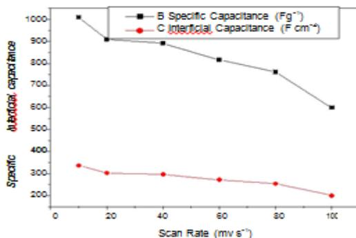
Fig 7. Variation of specific and interfacial capacitance with scan rate.
