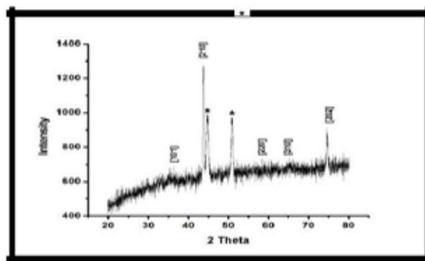
Fig 1. X-ray Diffractogram for RuO<sub>2</sub> thin films on stainless steel substrate.
