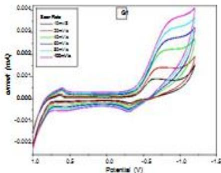
Fig 6. CV of RuO<sub>2</sub> with different scan rate.
