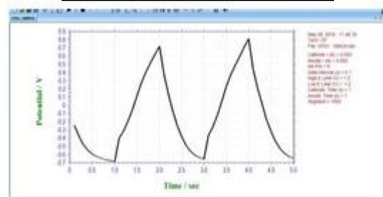
Fig 8. Galvanostatic charge-discharge curves of RuO<sub>2</sub>.
