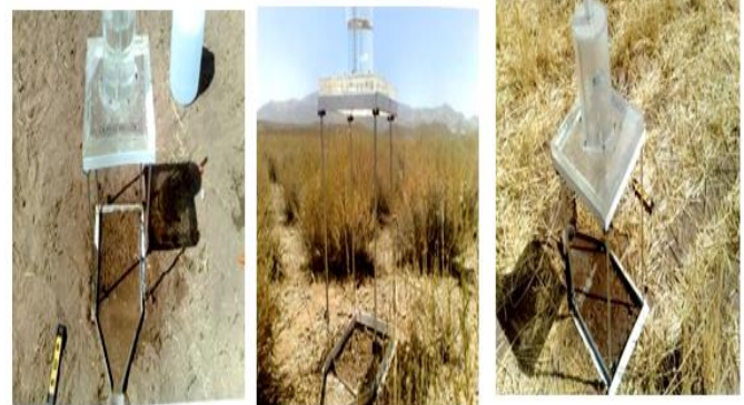
Figure 2. Correct placing of the rainfall simulator device in uses of rainfed, pasture and abandoned rainfed.
