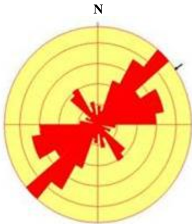
Axial (non-polar) data; No. of data = 146 Sector angle = 10°; Scale: tick interval = 3% [4.4 data] Maximum = 14.4% [21 data]; Mean Resultant direction = 056-236 [Approx. 95% Confidence interval = ±15.7°]
