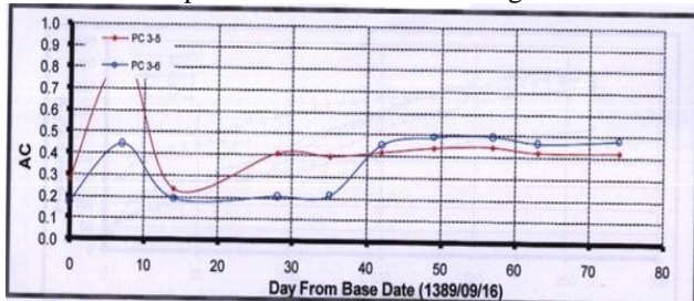
Figure 8. The arching coefficient variation curve, over time for the total pressure cells PC3-5 and PC3-6 [9].
