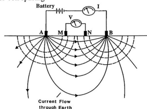
Figure 2. Typical electrode configuration for Schlumberger array.
