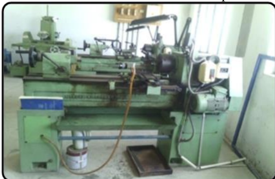
Fig.2. Kirloskar model Turn master 35 centre lathe.
