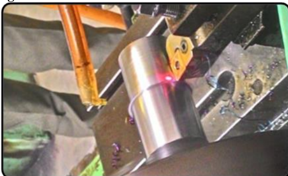
Fig.3. Cutting fluid dropping on cutting zone.
