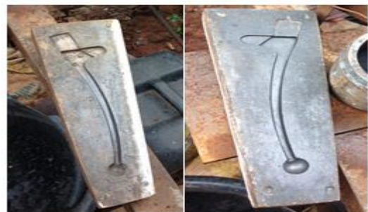
Figure 1. Pattern for motorcycle brake lever.
