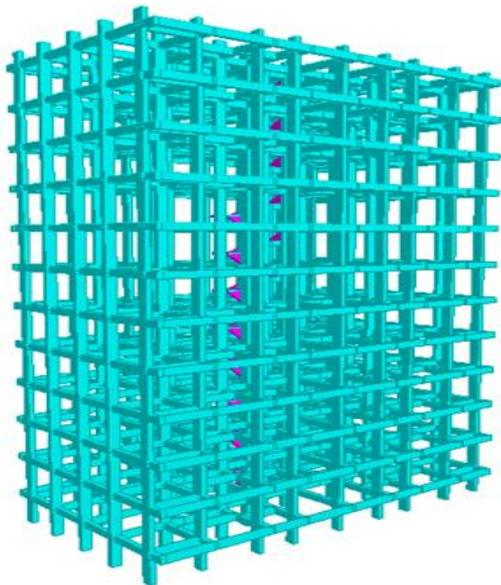
Fig. c. 3D Rendered View of Structure with Isolated Footings Modelled in STAAD Pro.
