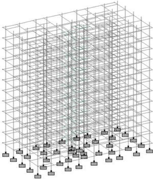
Fig. b. Structure with Isolated Footings Modelled in STAAD Pro.
