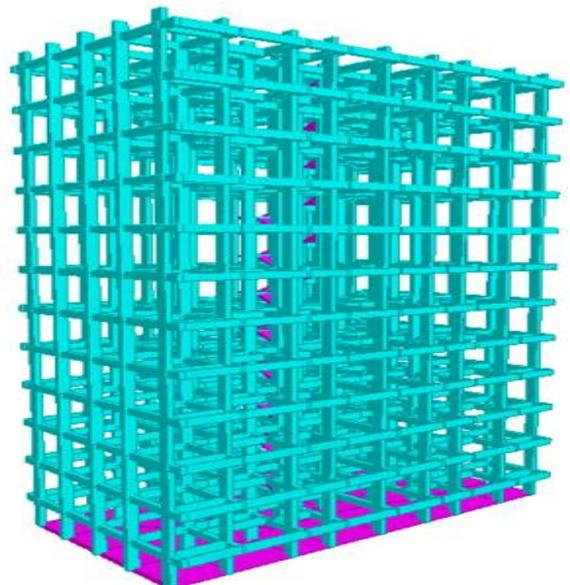
Fig. g. 3D Rendered View of Structure with Raft Footings Modelled in STAAD Pro.
