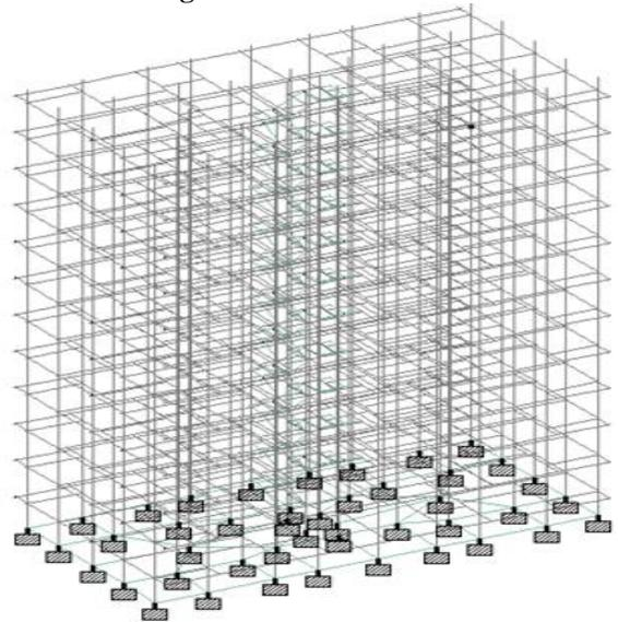
Fig. f . Structure with Raft Footings Modelled in STAAD Pro.
