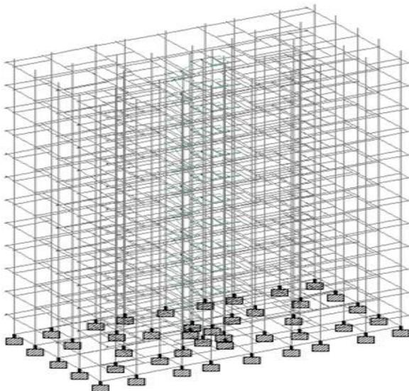
Fig. d. Structure with Strap Footings Modelled in STAAD Pro.
