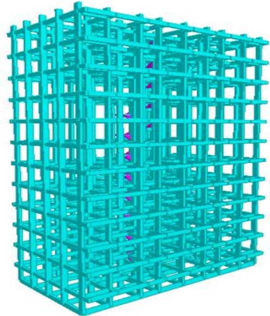
Fig. e. 3D Rendered View of Structure with Strap Footings Modelled in STAAD Pro.
