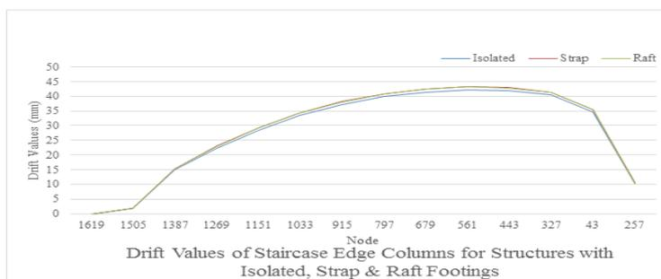
**Fig. j. Graph Showing Comparison between Drift Values of Outer Edge Columns for Structures with Isolated, Strap & Raft Footings.**
