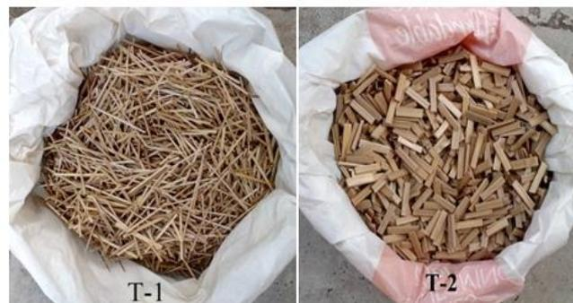
**Fig 2. The two types of Bamboo fibres.**
