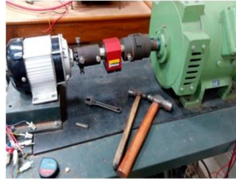
Figure 4. Coupling of dc generator for electric loading.
