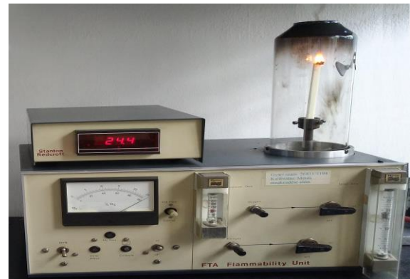
Fig 2. Mechanism Limiting oxygen index instrument (BorsodChem Zrt.).
