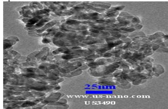
Fig 4. SEM image for anatase TiO<sub>2</sub>.
