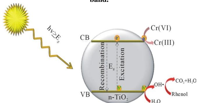
Fig 3. Showing the simultaneous mineralization of an organic pollutant reduction of an inorganic ion, Cr (VI) to Cr (III).
