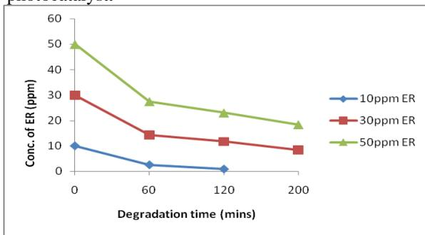
**Fig 11. Effect of Contact time. Reaction condition: pH = 6.63; 8W UV bulb, catalytic loading = 2g/L.**
