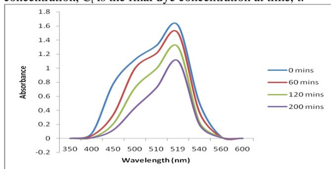
Fig. 8. Absorbance curve for the photodegradation of 50ppm ER. Reaction conditions:  $\text{TiO}_2 = 2\text{g/L}$ ; 8W UV light; pH = 6.67
