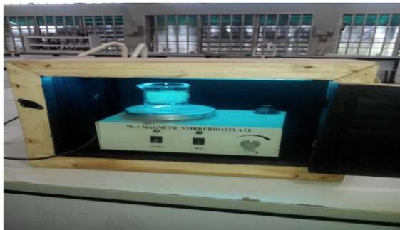
Fig 7. Showing the photoreactor and light source used in the research.
