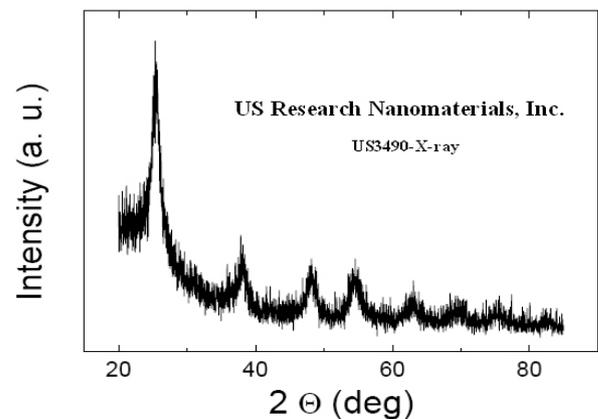
Fig 5. XRD pattern for anatase TiO<sub>2</sub>.
