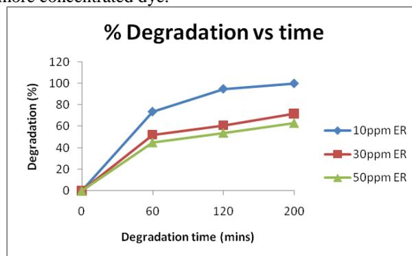
Fig 9. Influence of Initial Concentration on degradation efficiency. Reaction conditions: catalytic loading = 2g/L; 8W UV light, pH = 6.63.
