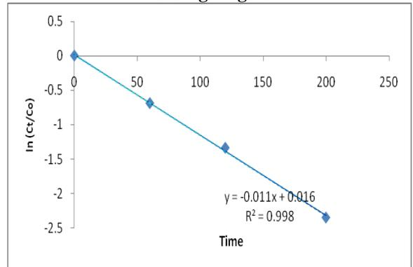
**Fig 13. The pseudo-first order kinetics plot for photodegradation of 10ppm ER.**
