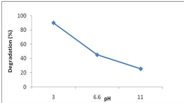
**Fig 10. Effect of pH on degradation efficiency. Reaction conditions: Dye conc.= 50ppm; catalytic loading = 2g/L; reaction time = 60 mins; 8W UV bulb.**
