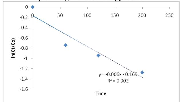
**Fig 14. The pseudo-first order kinetics plot for photodegradation of 30ppm ER.**
