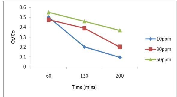
**Fig 12. Kinetics of the degradation of Eosin red dye. Reaction conditions: pH = 6.63; 8W UV bulb, catalytic loading = 2g/L.**
