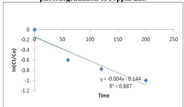
**Fig 15. The pseudo-first order kinetics plot for photodegradation of 50ppm ER.**
