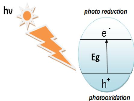
Fig 2. Showing to transfer of electrons from the valence band to the conduction band giving a hole in the valence band.
