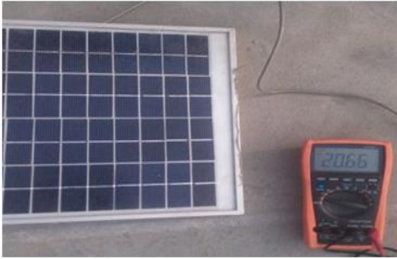
Fig 7. Output voltage of solar panel for charging the battery of the vehicle.
