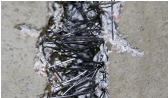
Fig 7. Steel fibres in concrete.
