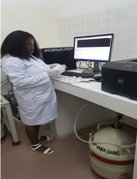
Figure 4. Borehole Water Samples analysis using High Pure Germanium detector in the lab
