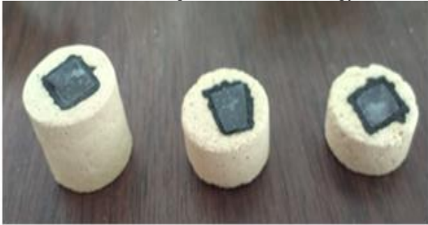
Figure 3. Pellet surfaces with copper after heat treatment at 1100°C.
