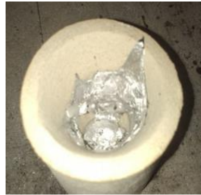
Figure 11. Aluminum melting in C4 crucible.
