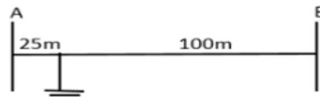
Figure 6(a). Close End Fault.
