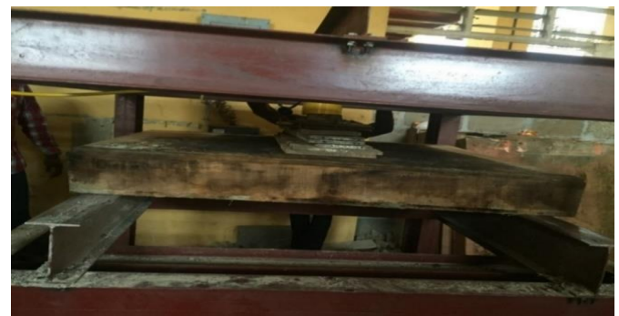
Plate 1. Positioning of composite slab.
