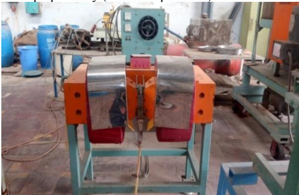
Figure 2. Boxmag High Intensity Magnetic Separator
