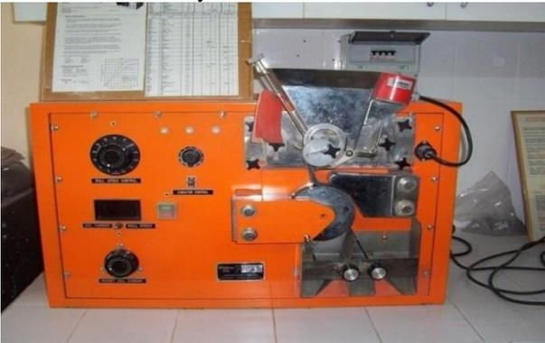
Figure 1. Dry Carpco Magnetic Separator
