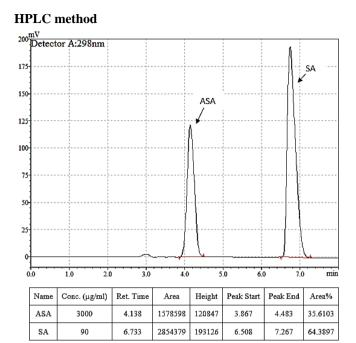
Figure 4. HPLC chromatogram of synthetic mixture of ASA 3000 & SA 90 ( $\mu$ g/ml) at  $\lambda$  298 nm using mobile phase mixture of: 40% of acetic acid 1% (v/v) aqueous solution and 60% methanol.
