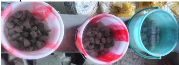
Figure 2. Recycled coarse aggregates in water
