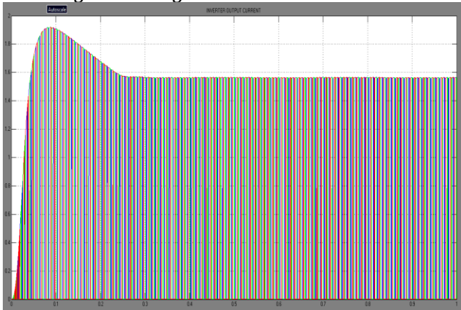
Figure 9. Current wave form of NPC inverter
